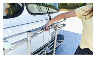
8. Stow the rack (if empty) – If no other bikes are on the rack and no one else is waiting to load, return the rack to the upright (locked) position and signal the driver when it's clear to leave.
