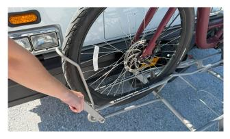
4. Secure with support arm – Pull the support arm up and over the front tire until it rests firmly against the tire. Board the bus when finished.
