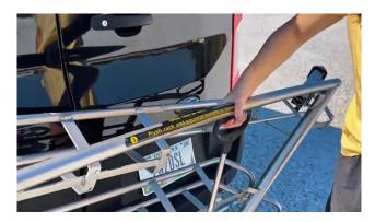
2. Lower the rack – If the rack is stowed upright, squeeze the latch handle to release. Then fold the rack down while holding your bike with your other hand.
