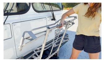
2. Lower the rack – If the rack is stowed upright, squeeze the release handle and pull the rack down.
