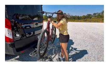
3. Place your bike – Lift your bike and set the front wheel into a labeled wheel slot (front wheel placement ensures easier loading/unloading).
