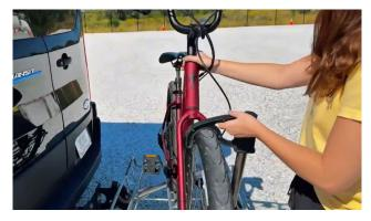
4. Secure with support arm – Pull the support arm hook up and over the front tire, placing it between the tire's highest point and the head tube. Ensure it's firm.
