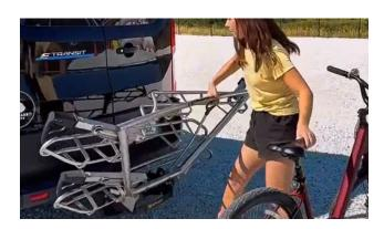
8. Stow the rack (if empty) – If no other bikes remain and no one is waiting to load, fold the rack back into the upright (stowed) position until it locks. Step back to the curb with your bike.
